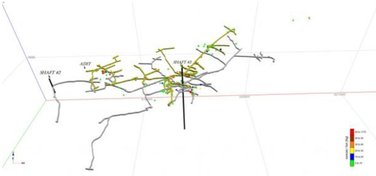
*View looking North through Castle No 3 Shaft showing Level 1 underground workings with grade points from historic drill holes (to date, from Level 1 only). Legend is the grade in ounces/ton Ag*
